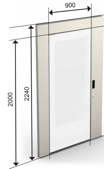
Example with door opening height 2000 mm.
